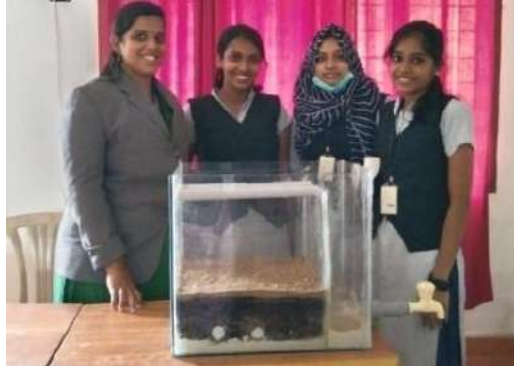
Rapid Sand Filter using Rice Husk and Groundnut Shell
